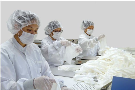
Fig. 12 The laying room in the Ostseewerk (Baltic plant). There the wipers are individually tested and packaged in the ISO class 5 cleanroom by Colandis in Kahla
