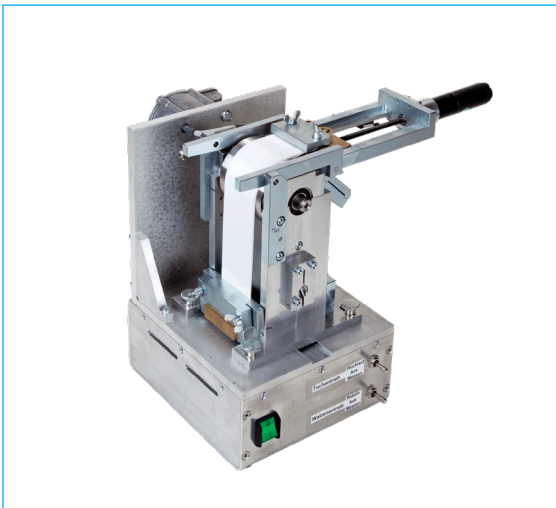
Fig. 6 Rotary wiping simulator Mark III according to Labuda/Schöttle to determine the cleaning effectiveness of different wipers.
